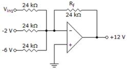
(b) Explain how an operational amplifier can be used as summing amplifier.
